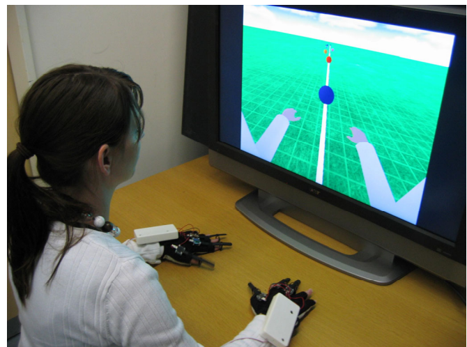
Fig. 1: The experimental setup with the data gloves and the screen with the presented interactive game
